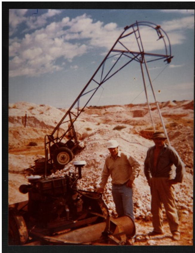
This bucket loading machine is typical of those used by many miners on the Andamooka and surrounding fields.
